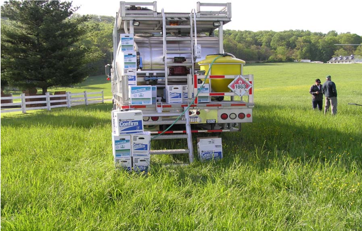
The truck was used to refill the spray tank, helicopters land on the top deck where the filling occurs.
